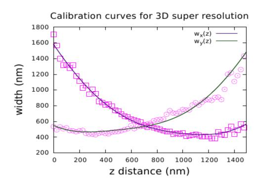
A set of cylindrical lens is introduced in the light path of image to distort the spots from circle to ellipse. The widths  $w_x \& w_y$  depends on the vertical position of the molecule. As a result, we can use the calibration curve to determine the z coordinate for the given  $w_x \& w_y$ .
