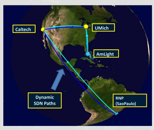
Successful Multi-domain Dynamic Paths using OSCARS, NSI with SDN as south bound. Moving forward to integrate with multi-domain Software Defined Exchanges (SDX)
