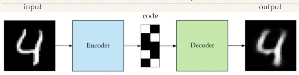
An AE consists of 3 components:
