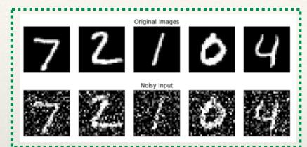
The input to the dAE is the noisy data. The expected target is the original noise-free data
