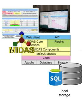
DAQ system of the CYGNO detector, that uses MIDAS framework to control it.
