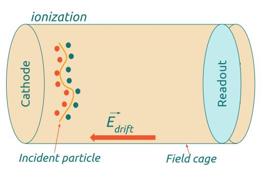
The operation principle of a **TPC gas detector readout** by a high-granularity **sensor** is the following:
