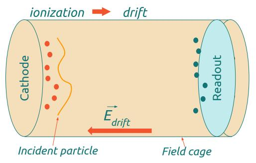
The operation principle of a **TPC gas detector readout** by a high-granularity **sensor** is the following:
