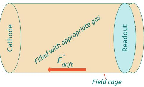
The operation principle of a **TPC gas detector readout** by a high-granularity **sensor** is the following:
