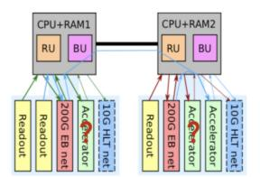
GPU-equipped event builder PC, with traffic of all three readout cards.
