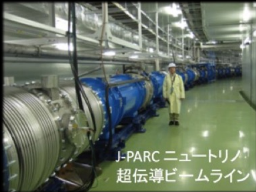
J-PARC neutrino super-conducting beam line
