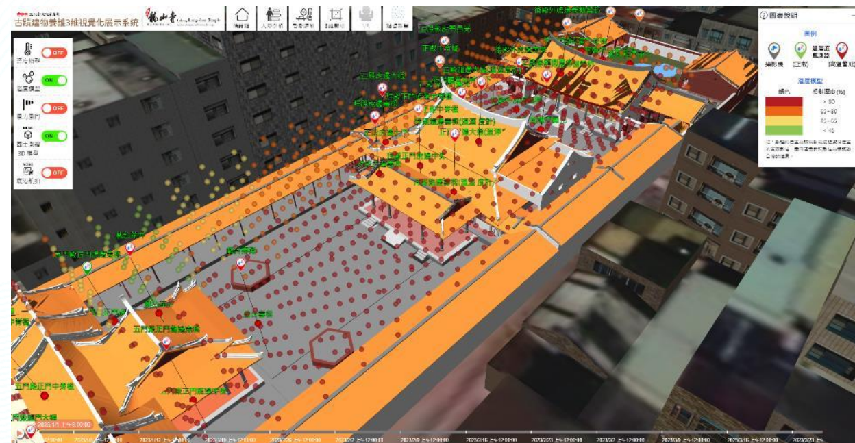
Digital twin of ancient monument model, with temperature and humidity monitored inside
